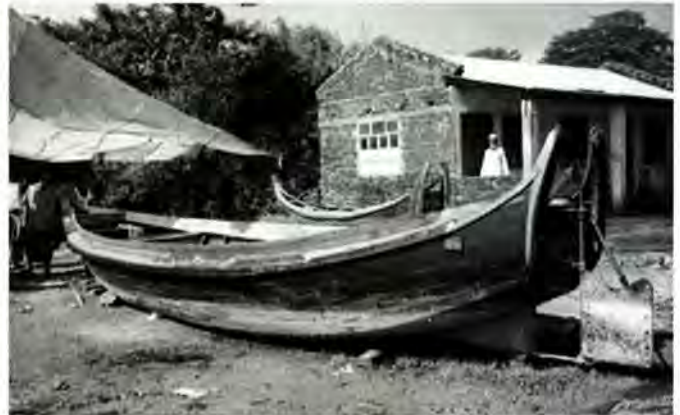
Fig. 4.19 A sampan fitted with an iron rudder under repair
