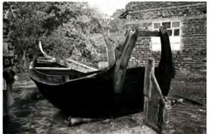
Fig. 4.20 A sampan fitted with a wooden rudder under repair
