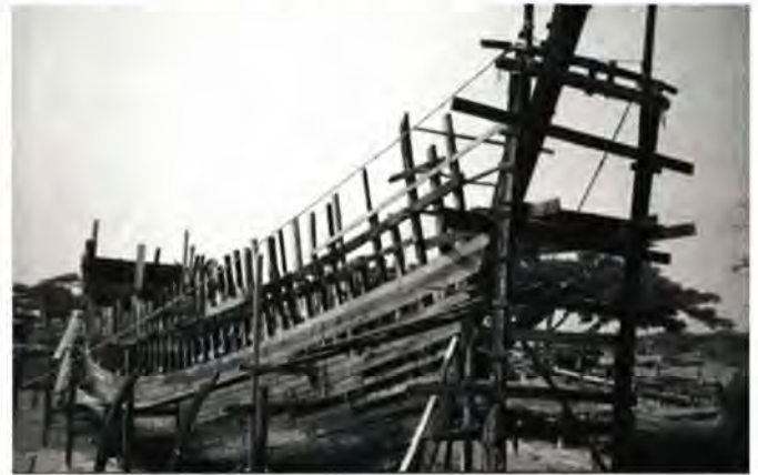
Fig. 4.13 A skeleton-built boat under construction, Cox's Bazar
