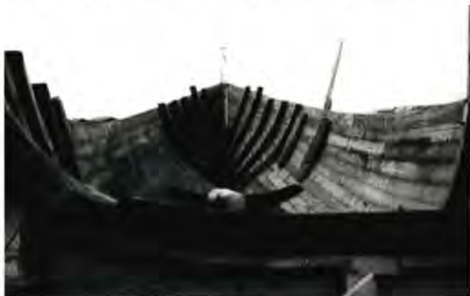
Fig. 4.16 A shell-built boat under construction at Digha
